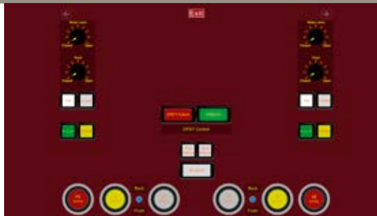
4. Configurable top plate-mimicking touchscreens provide a realistic adaptation to the particular vessels' console components
